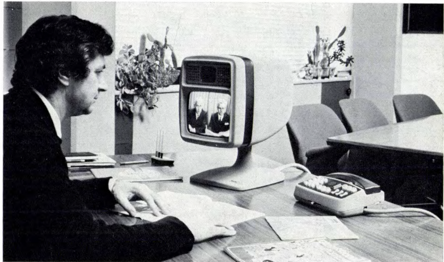
Fig. 5. Video-telephone station set designed by Philips Telecommunication Industries (PTI) for use in the national experimental network. Like the set developed at Philips Research Laboratories (fig. 4) it consists of three units. The technical differences are only minor.
