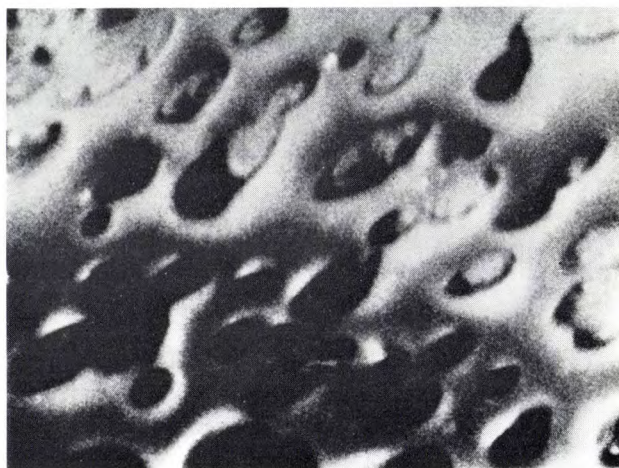
Fig. 5. An intermediate stage in the charge-compensation process (see fig. 4c ). The areas inside the domain walls are still partly black, indicating that charge compensation is not yet complete.
