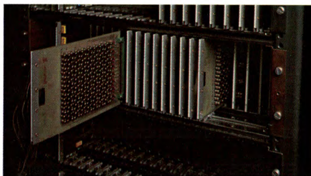
Fig. 18. Detail of the experimental video-telephone exchange at Philips Research Laboratories, Eindhoven. Ten printed-wiring boards carry the entire P-N-P-N switching network, which consists of discrete P-N-P-N elements. The pulled-out board carries a 16 \times 8 matrix; at each crosspoint there are two small metal 'cans', one for the P-N-P-N element and one for the control circuit.
